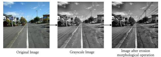
Fig. 2 Road damage image transformation during preprocessing stage
